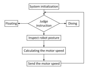
Fig. 3. The software design process of the Robot attitude control system
