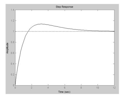
Fig. 10. The transfer function–roll channel
