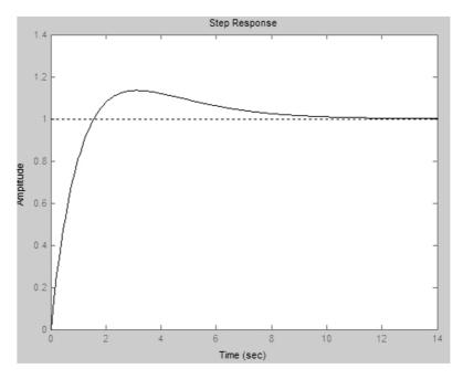
Fig. 11. The transfer function–pitch channel
